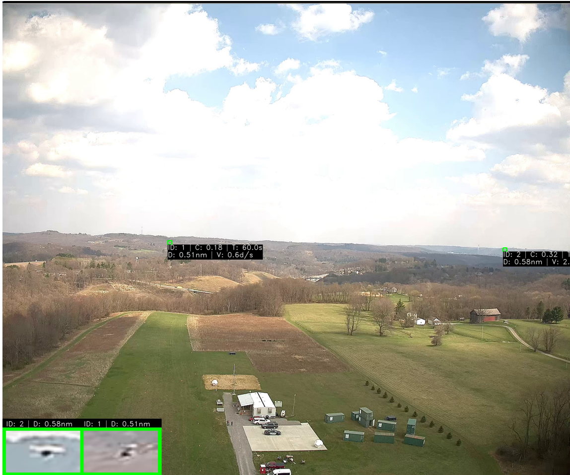
Figure 5.2: TartanX6C drone-helicopter encounter sequence with relative velocity of \sim 40\text{m/s} . This shows an example of below-the-horizon detection. The detector also picks up the hovering filming drone of the encounter on the right.
