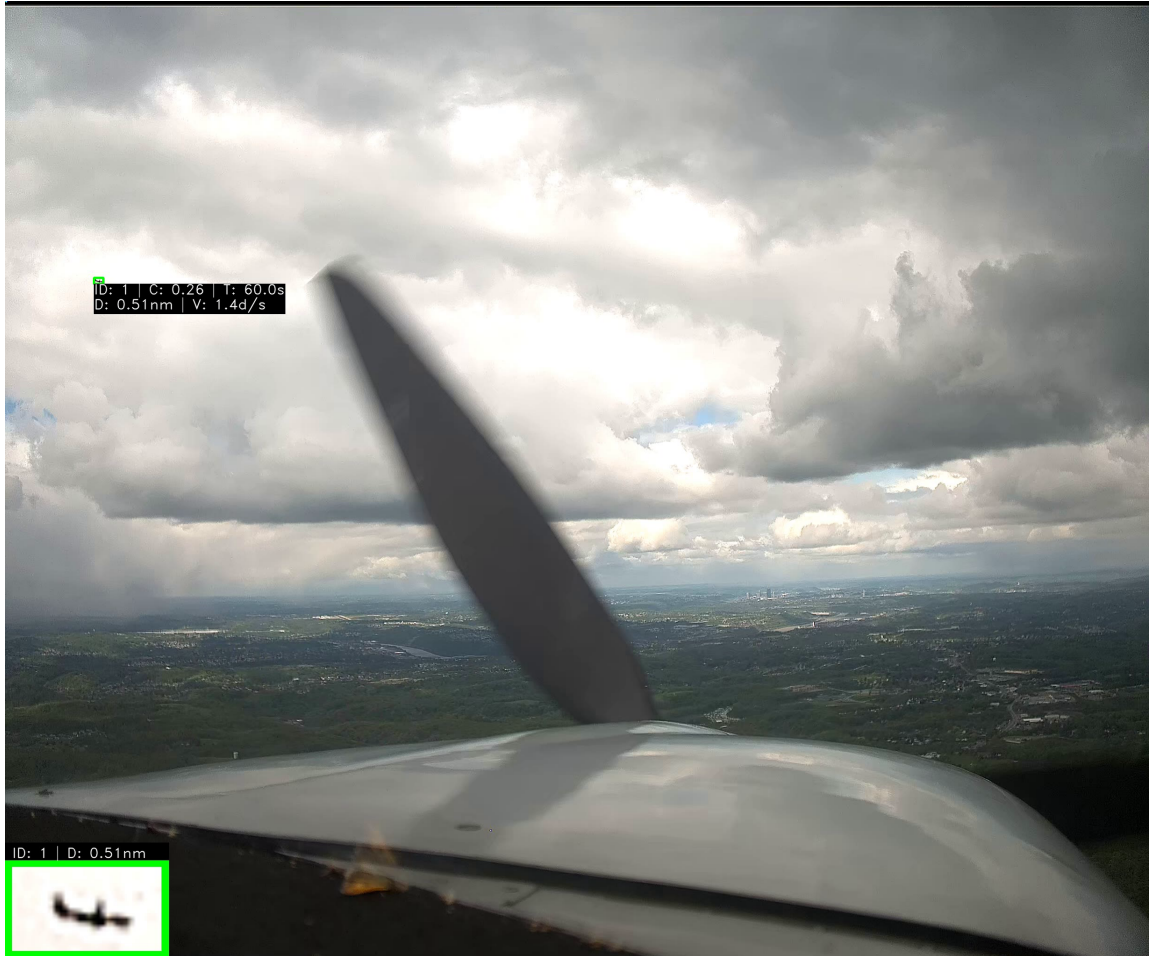
Figure 5.3: TartanX6C in-flight Cessna sequence capturing another aircraft in a non-collision course.
