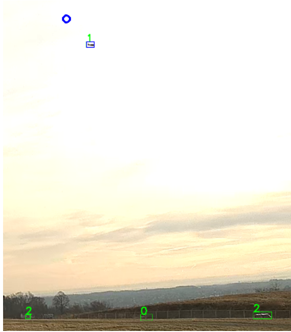
Figure 3.4: Visualization of auto-labeling pipeline. The reprojected point based on ADS-B is shown in the blue circle. The bounding boxes are predicted by the detector and it can be in the bottom of the image, there are false-positives. Using the reprojected point, we can reject those false-positives for new ground truth label generation (chosen label is highlighted in the blue).
