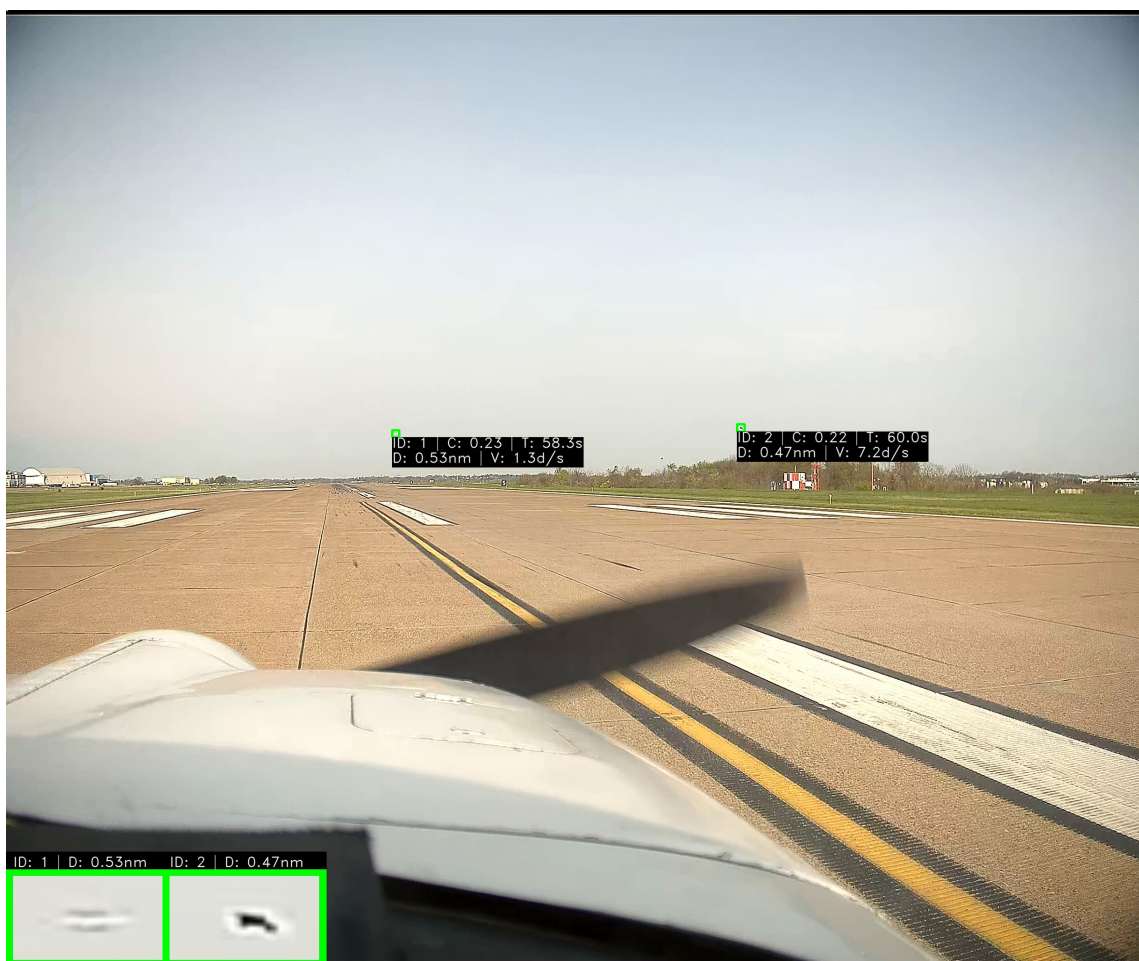
Figure 5.4: TartanX6C in-flight Cessna sequence chasing another aircraft during takeoff. Bird detection is observed on the right as well.
