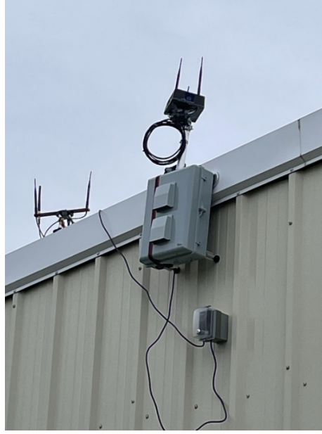
Figure 3.3: Static 4-camera setup mounted on a hangar at Allegheny County Airport (AGC). This data collection setup is remotely monitored and can automatically capture aircraft data (ADS-B + video) from sunrise to sunset everyday.
